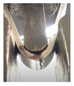
Fracture test: The joint is fractured to identify the internal imperfections such as porosities, cracks, lack of fusion, lack of penetration and solid inclusions on the fracture surface.
